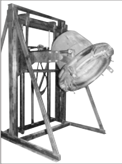
▲ This 6,000 lb. capacity 180° Container Inverter is designed to lift and empty special processing vats.
