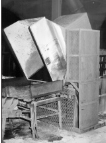
▲ A 1,000 lb. capacity Extended Height Dumper is used at a galvanizing plant to transfer small parts from a 12' deep cooling tank onto a sorting conveyor.
