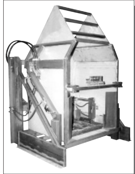
▲ This stainless steel Rolo-6000 is designed with a custom hydraulic container latching mechanism designed for holding special containers during the dumping process.
